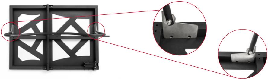
3. Tighten the four screws with a 4 mm torque wrench (tightening torque 9.5 Nm).
